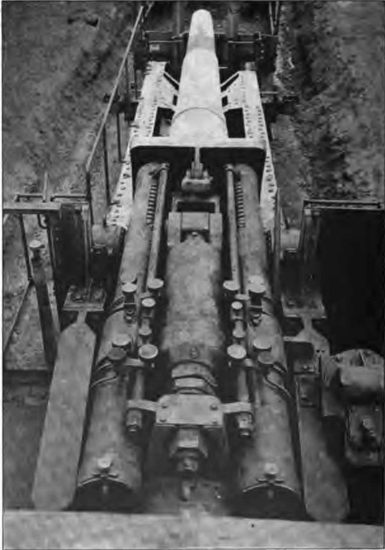
CRADLE, RECOIL CYLINDER, AND SPRING RECUPERATORS OF THE 210-MM. GERMAN GUN MOUNT.
